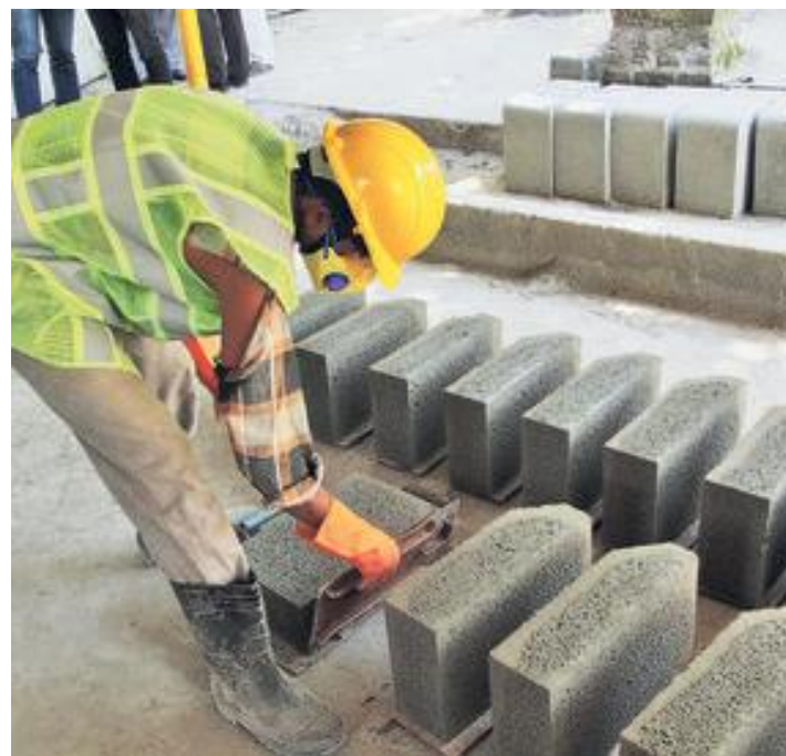
A worker demoulding kerb-stones made with the revolutionary cement
